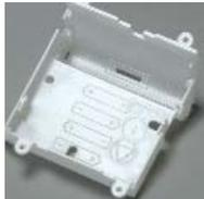
Pair of dishwasher components (grey and natural) produced for functional testing.
