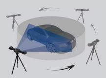
Flexible measurement volume that can be easily and dynamically extended without loss in accuracy or conventional leapfrogs.
