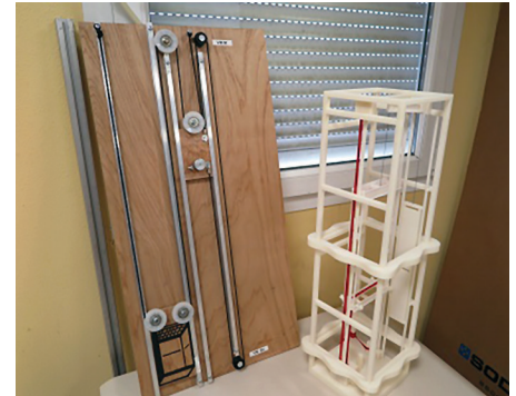
The 3D printed elevator training model (right) is lighter than the previous wood-mounted version (left).
