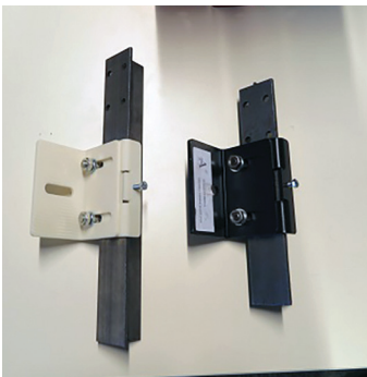
3D printed prototype part (left) is tested for form, fit and function before the final part (right) is produced.
