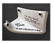
Front bumper drill fixture used to test the design.
