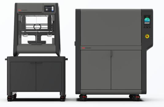
1. Unlike comparable metal 3D printing systems, Studio System<sup>™</sup> 2 eliminates loose metal powders and features a two-step process (no solvent debind required) and features Separable Supports<sup>™</sup> technology with strategic splits for hand-removable supports, hot swappable cartridges and removable printheads to make material changes easy, and a fully software-controlled workflow.
