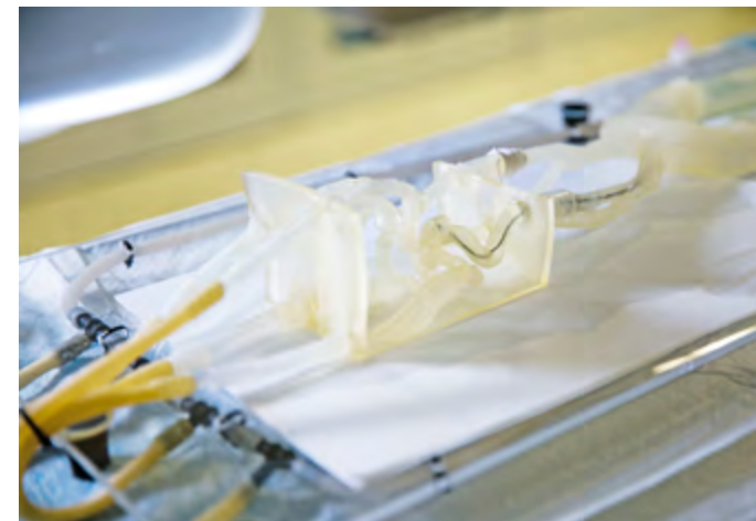
The clear, flexible material of this vascular model was used to assess the feasibility of a proposed aneurysm treatment, before operating on the patient.
