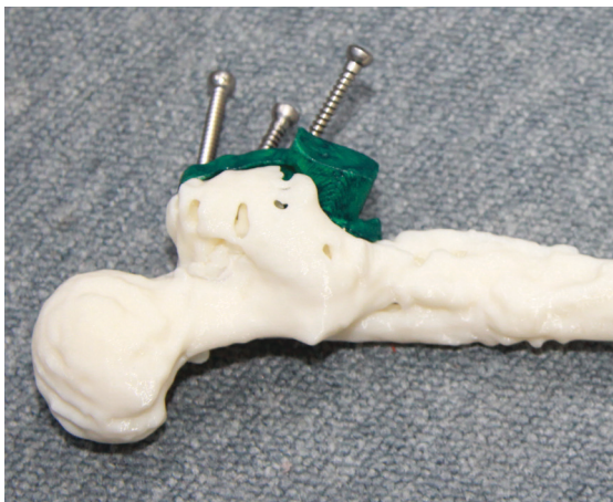
Figure 9 - A 3D printed bone model using a customized guide for pre-surgical planning.
