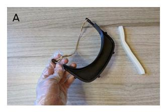
Take the 3D printed part and dip it into the prior mixed solution. Let the remaining liquid drip off and set to the side. Take either an elastic- or rubber band and tie it to the end of either side of the visor.
