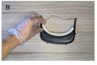
Prepare the print and the liquid glue. Add some glue to the inside of the rim of the 3D printed part. Take the foam material and gently press the foam material onto the inside of the 3D printed part.
