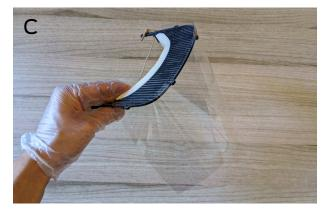
Take a marker and mark the points on the PVC where you need to punch a hole to attach the PVC to the hooks of the 3D printed visor.
