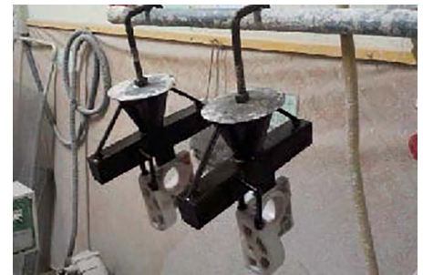
Figure 27: Part with added venting.
