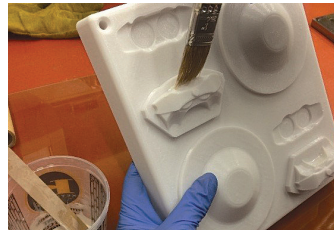
Figure 4 – Sealing particular areas of the tool will promote a more uniform formed sheet thickness.
