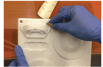
Figure 3 – Sanding will improve the surface finish of the molded part.
