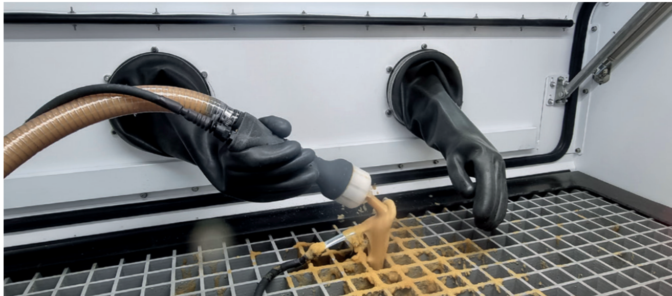
Projection system - eBlast working by electro-blasting solution
