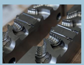
The final roughness achieved with this process is very low -Ra (final) < 0.01  $\mu m-$  in short cycles while avoiding undesired side effects on the surface.
