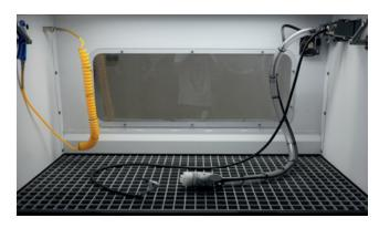
The work area has been designed to hold 300 kg and a maximum piece volume of 1,000 x 500 x 500 mm. Heavy parts can be placed easily with a bridge crane as the cabinet includes front loading and top loading doors.
