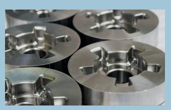
Parts with cavities and narrow spaces such as blind holes, slots, corners and occluded areas can be treated, as eBlast uses a fluid instead of a granular material, and is able to focus the media stream towards the target area from a very short distance.
