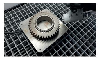
The turntable system increases comfort, and productivity while decreasing the overall operator's fatigue. By placing the part on the turntable, and manually spinning it while electro blasting it, saves time and effort from lifting and turning heavy parts.
