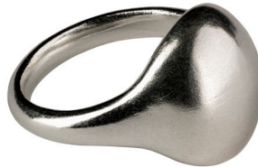
After Sintering + Pin Finishing
