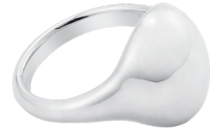
After Sintering + HIP + Polish
