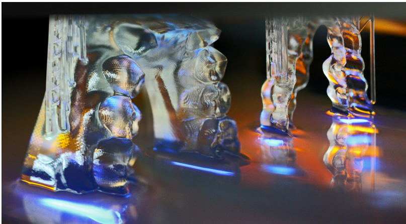
— DLP printing is used widely for precision medical applications. E-Guide, shown here printing on a Desktop Health printer, is a biocompatible certified Class I material used for precision surgical drill guides used for implant surgery.
